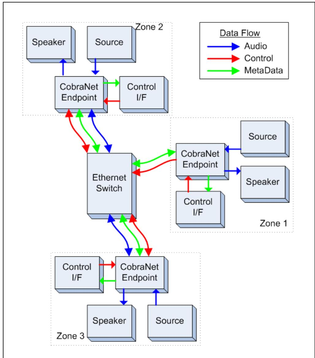
The main difference between this and the previous strategies is that there is no longer a central control unit. All the intelligence has been moved into the endpoint and each can function on its own.
